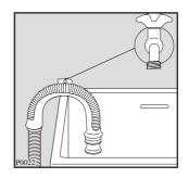
If the machine is permanently plumbed in, hook the end of the hose into a standpipe installed for the purpose. The standpipe must have an internal diameter of at least 40mm in order that there is an air gap between the drain hose and the standpipe. Make sure, that it is designed in such a way, that the end of the drain hose cannot be covered with water.
